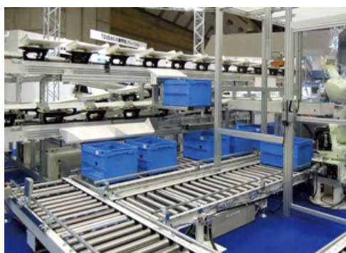
LiniSort S-C (combines robots to raise the level of automation)
