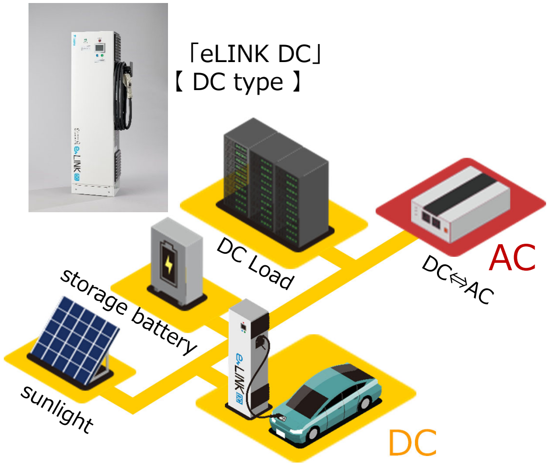
High efficiency through DC connection
