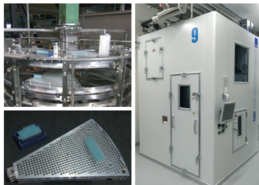
Tsubaki Labo Stocker®, capable of storing approximately 50,000 samples at the ultra-low temperature of -150°C
