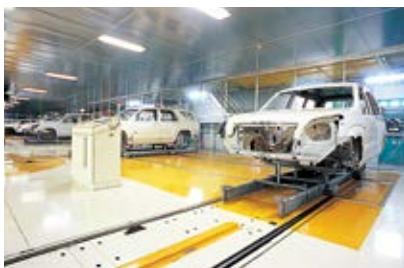
■ Conveyance system for automobile manufacturing line
